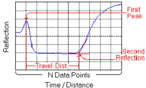
**Figure 1:** Basic principles used by WinTDR for analysis of a waveform.
